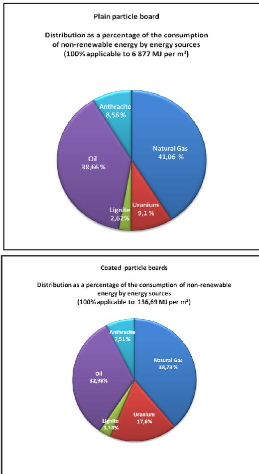
A more detailed analysis of the consumption of non-renewable energy in manufacturing 1 m<sup>3</sup> of plain particle board and 1 m<sup>2</sup> of melamine-coated particle board (figure 3) shows that, in both cases, natural gas is used as source of
