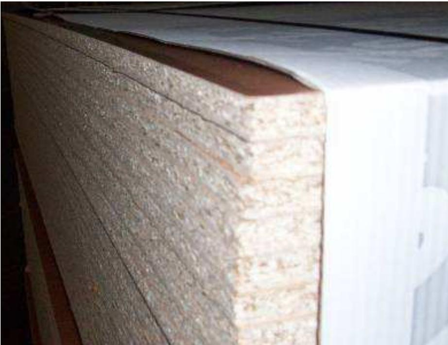
Figure 2: Finished product\_ melamine coated particle boards
