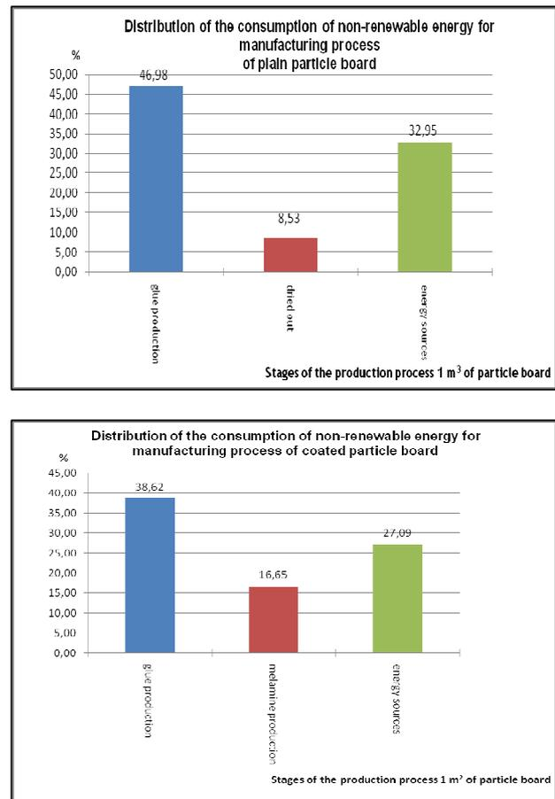
Figure 2 provides a level for the consumption of non-renewable energy per process stage, in manufacturing plain particle boards and melamine-coated boards.
