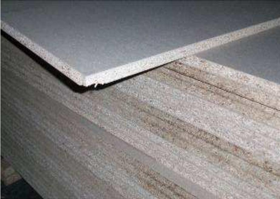
Figure 1: Finished product\_ plain particle boards
